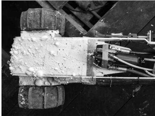
*The Q-Bot is sent into the under-floor void in older homes to scan the area and squirt insulation*
